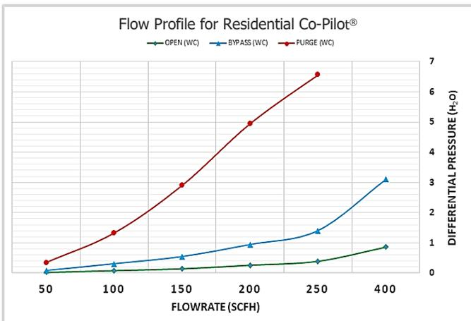
Flow testing done with a residential meter set (20LT meter and regulator), 40k BTU burners, and 3x pilot lights.
