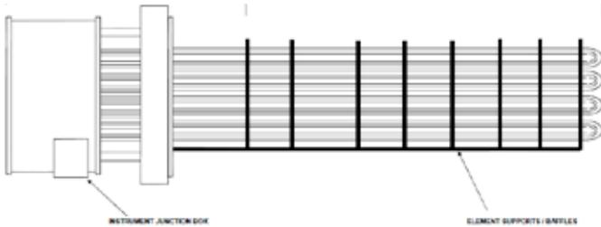
Example of electrical Gas Heating to prevent condensate creation after the gas temperature reducing at the pressure reducing valves for the joule-Thompson effect.
