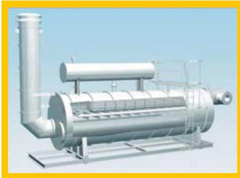
The heater shell contains the fire-tube that allows a rapid heat transfer (both radiant and convective) from the flame to the hot medium. The heat is transferred from the bath to the coil / tube bundle and then safely to the gas or the oil.
